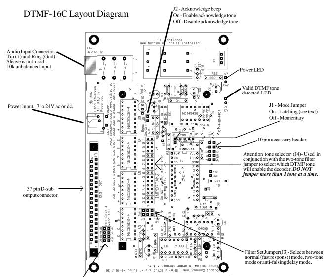
Hex data/Db-37 output jumpers/header Normally jumpered, can be removed (disabling the hex data outputs) so that the corresponding D-Sub pins (2, 3, 4, & 23) can be used by other assemblies in the product enclosure, like the optional Silencer.
