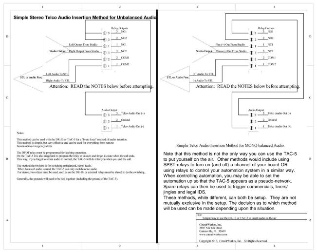
Switching of unbalanced stereo or balanced mono can be done using the onboard relay of the TAC-5. To switch stereo, balanced audio using the TAC-5, yiou would need a slave relay. Note that it is possible to program two relays on the TAC-5 to respond to the same codes. So, a small DPDT slave relay could be driven from K3 which could be programmed to respond to the same command as K2, thus providing four sets of contacts. Note that the slave relay will need its own power source.
