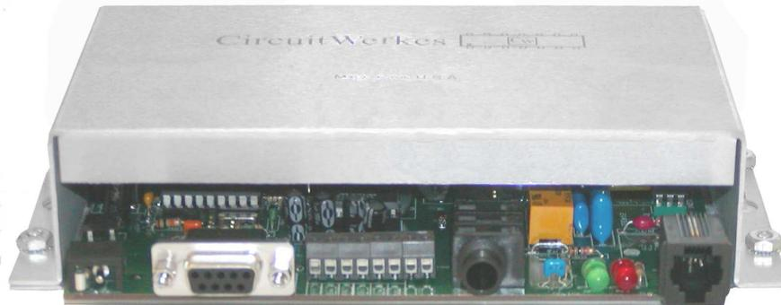
The DT-232 is an inexpensive dial-up remote control with amazing capabilities! It gives you DTMF access to four, user programmable relays that can be momentary, latching, etc. Relays can be programmed to respond to any DTMF tone or sequence.
