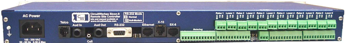
Figure 1. The back panel of the Sicon-8
