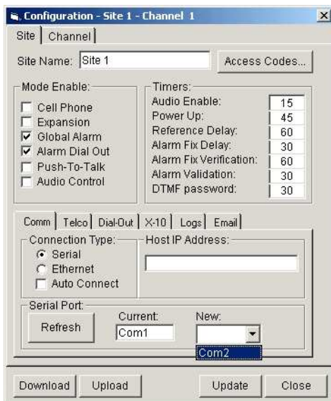
Left: Setting the com port. Above: Setting the hardware passwords
